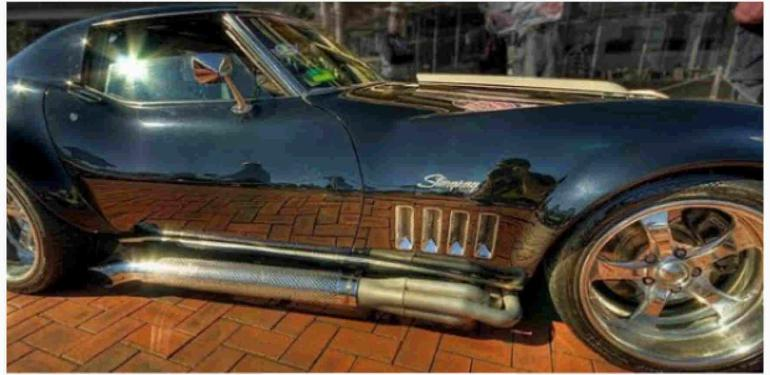
C3 Corvette Side Pipes The only C3 Corvette that had RPO N14 was the 69 Corvette.
